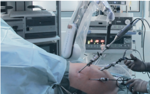
// The robotic arm Soloassist II in action: With the help of voice control, the surgical camera is guided by the surgeon to the right place and provides him with a perfect steady image.
