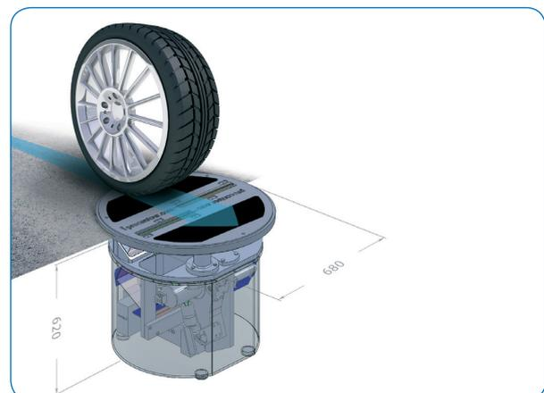
Image 2: Via laser diode-digital cameras, which are fit into shafts in the highway or troughs, tire treads depths can be captured and calculated in milliseconds by the integrated DIN rail PC, Kontron ThinkIO.
