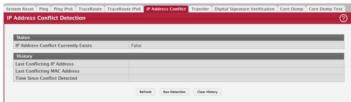
Figure 117: IP Address Conflict Detection
