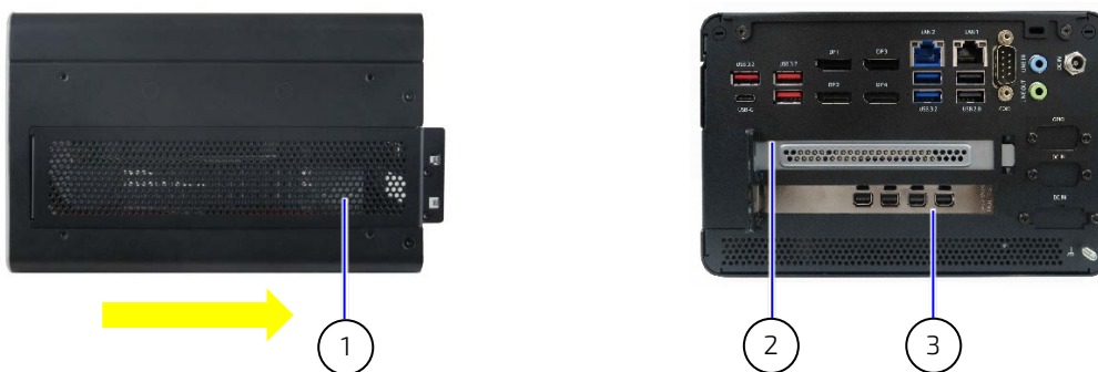
Figure 17: Removing Expansion Door
