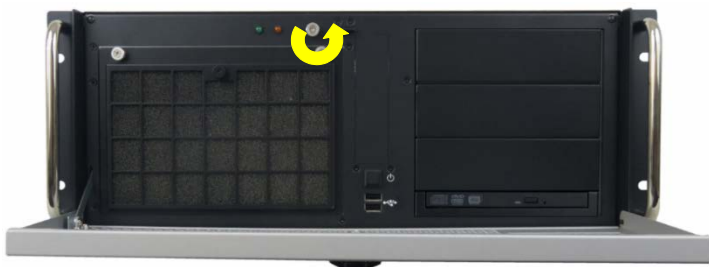
Figure 22: Loosening Knurled Screw (front panel)
